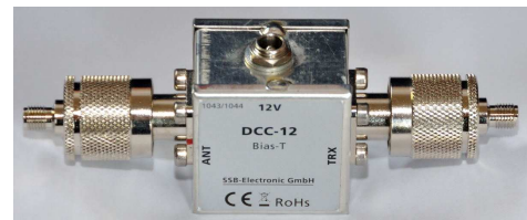
Fig. 52: The bias tee used for DC voltage supply of up to 12V
