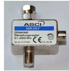
Fig. 54: An attenuator with a value of 0.5 dB up to 20 dB
